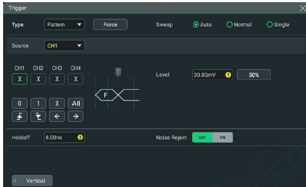
Figure 8.10 Pattern Trigger Setting Menu
