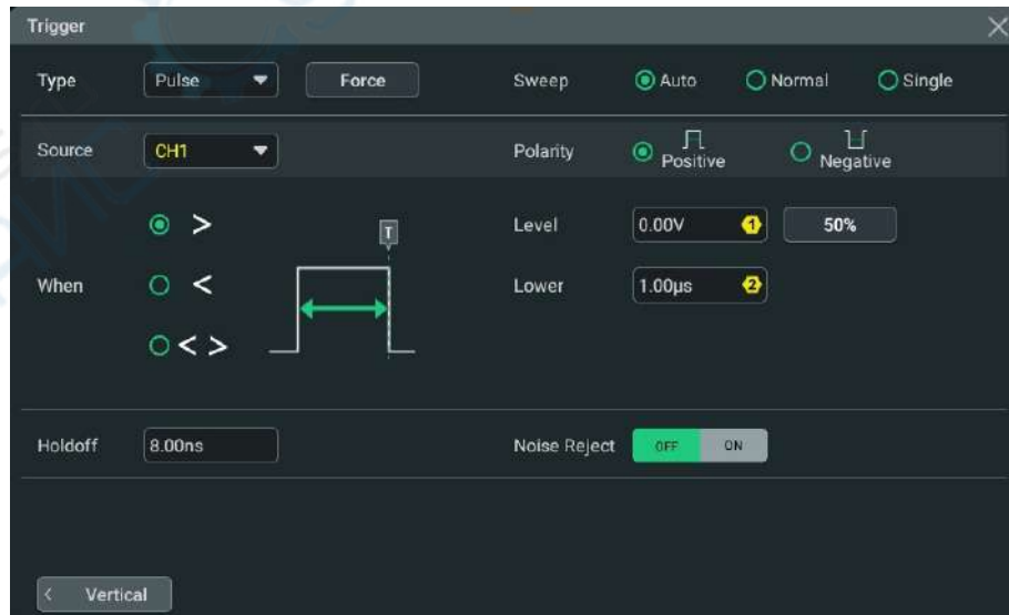
Figure 8.5 Pulse Width Trigger Setting Menu
