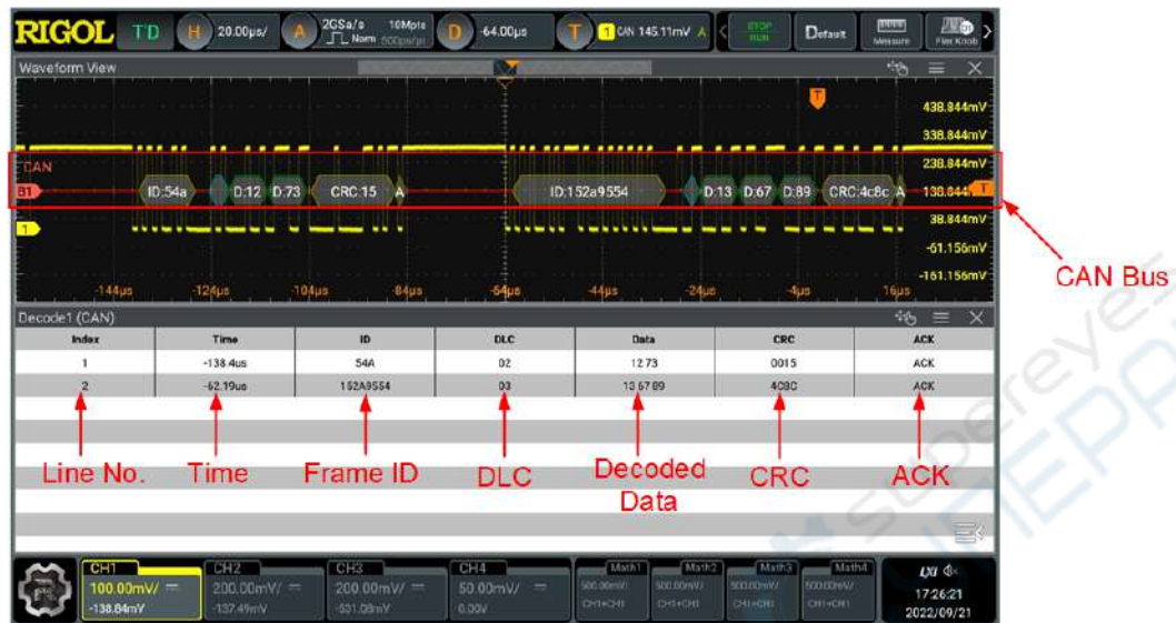
Figure 15.15 CAN Decoding Event Table
