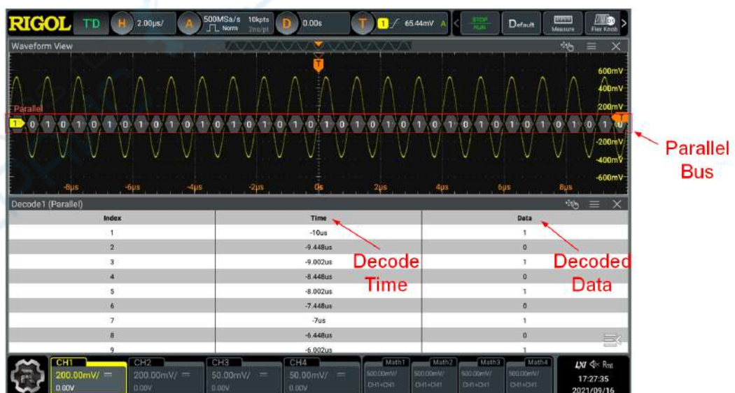
Figure 15.3 Parallel Decoding Event Table
