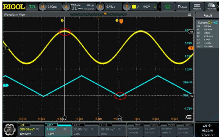
Figure 10.13 Track Measurement (after Horizontal Expansion)
