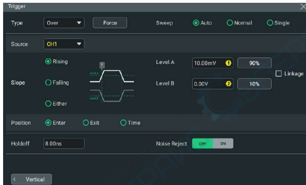
Figure 8.17 Window Trigger Setting Menu
