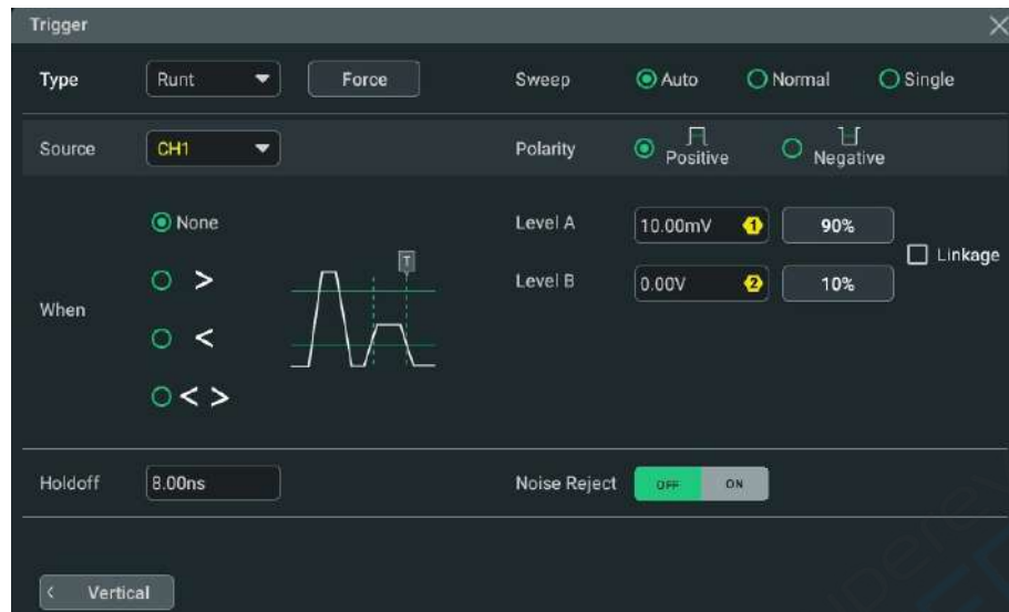
Figure 8.16 Runt Trigger Setting Menu
