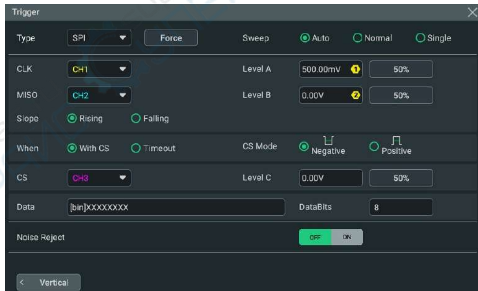
Figure 8.31 SPI Trigger Setting Menu
