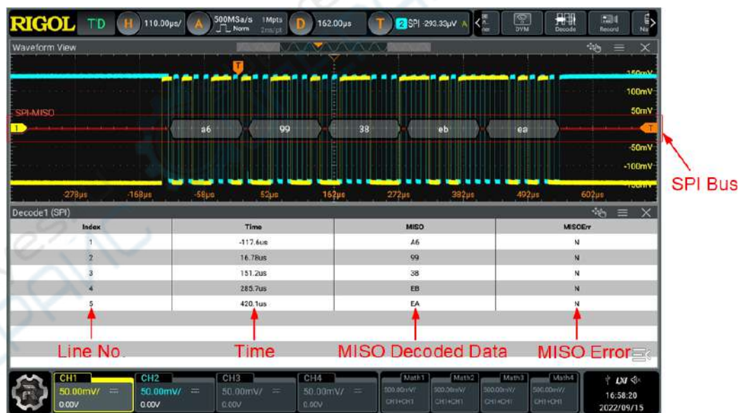
Figure 15.12 SPI Decoding Event Table
