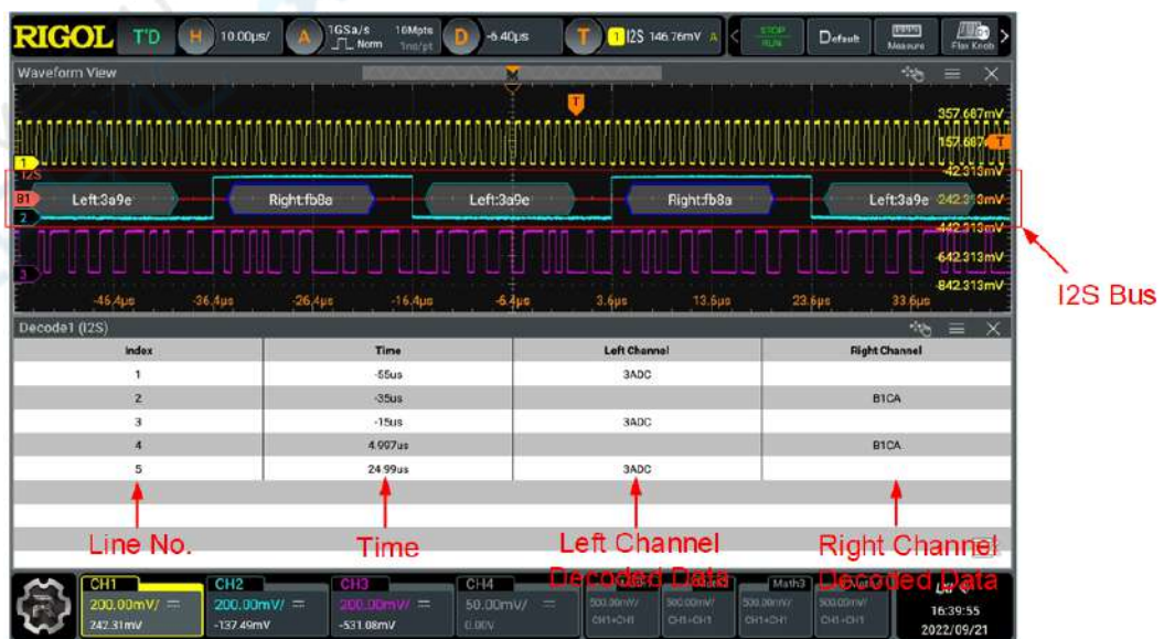
Figure 15.19 I2S Decoding Event Table
